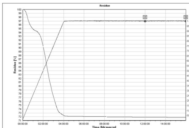
Fig. 2 Residual weight and temperature (°C) versus time (Hrs) for one sample in the prepASH129 furnace
