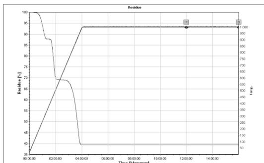
Fig. 3 The thermogram recorded for Calcium oxalate monohydrate with the prepASH129
